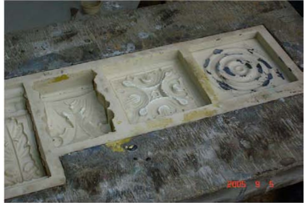
8. The mould of the architrave products.
