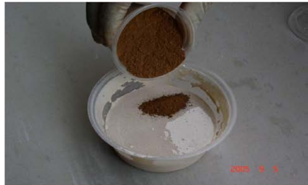
2. Grinded waste is mixed with inorganic composite binder.
