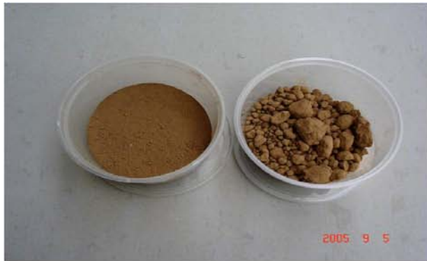
1. Lumpy and dry waste is grinded to powder and use as filler.
