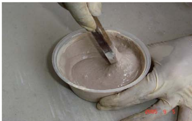
5. The grinded waste and inorganic composite binder must be mixed thoroughly.
