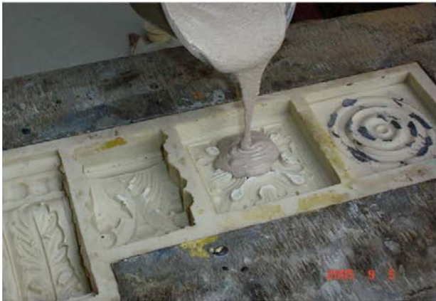
9. Pouring of final mixture into the mould.
