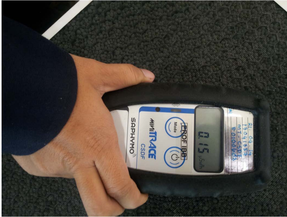
Test of radiation on Biowave Filter (0.15 \mu\text{Sv/h} )
