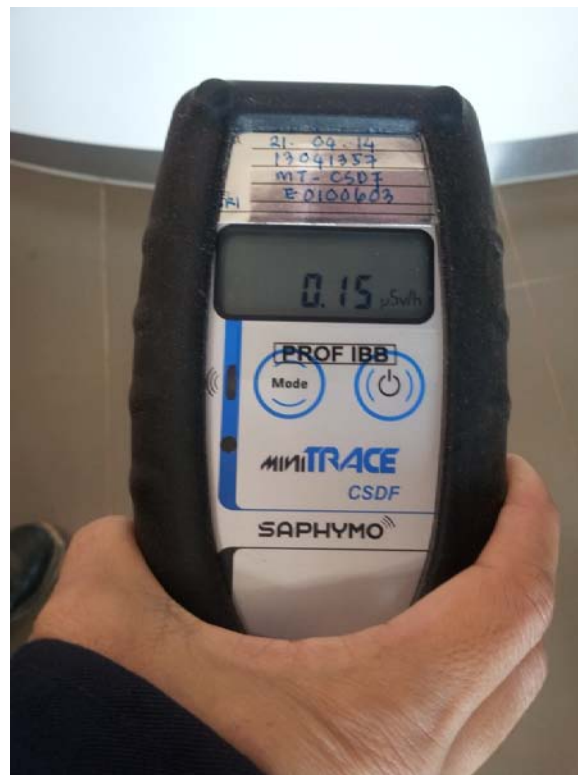
Test of radiation in ambient surrounding (0.15 \mu\text{Sv/h} )
