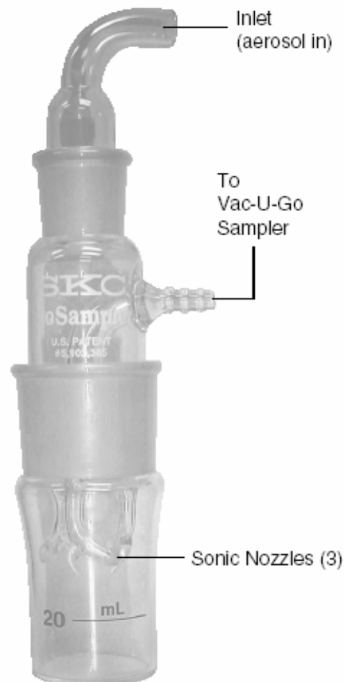
Figure 1. BioSampler with 20 ml vessel (5 ml vessel available)
